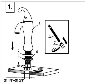
Make a mounting hole. Remove nuts (7) from mounting shanks (6). Install mounting shanks (6) and supply hoses (8) onto faucet body. Place hoses and shanks through mounting hole and slide faucet down until it rests on mounting surface.
