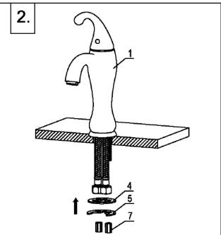
Slide gasket (4) and bracket (5) up over hoses and shanks and install under faucet body. Thread nuts (7) onto mounting shanks.
