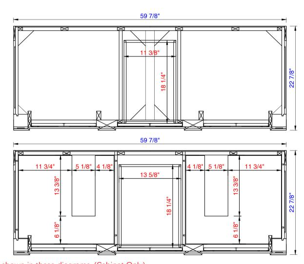
NOTE ONE: Countertops are not shown in these diagrams .(Cabinet Only) NOTE TWO: Internal Shelves (Shown) are designed to align with sinks in Ja
