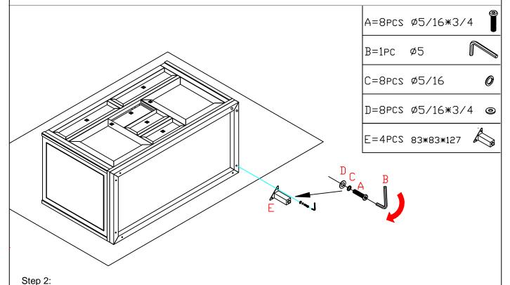
Attach the Legs to the Cabinet, insert the bolt (A) through the Spring Washer (C), Flat Washer (D) through into the pre-drilled holes at the bottom of Cabinet, then tighten the bolts using by Allen Wrench.
