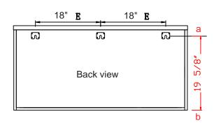
Step 1: Metal plates has been pre-installed to the back of cabinet, measure the distance between the bottom of the cabinet and point a.
