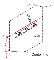
Step 2: Draw a horizontal line from the point a by using a leveler. (suggested H24 1/4" from floor to "a" line)
