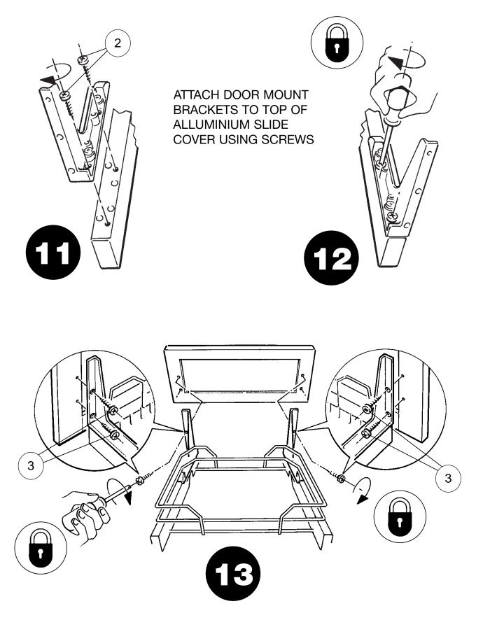
ATTACH BASKET WITH BRACKETS TO CABINET DOOR. BE SURE UNIT IS CENTERED SIDE TO SIDE AND AT THE PROPER HEIGHT TO ALLOW PROPER OVERHANG OF DOOR AT TOP AND BOTTOM.
