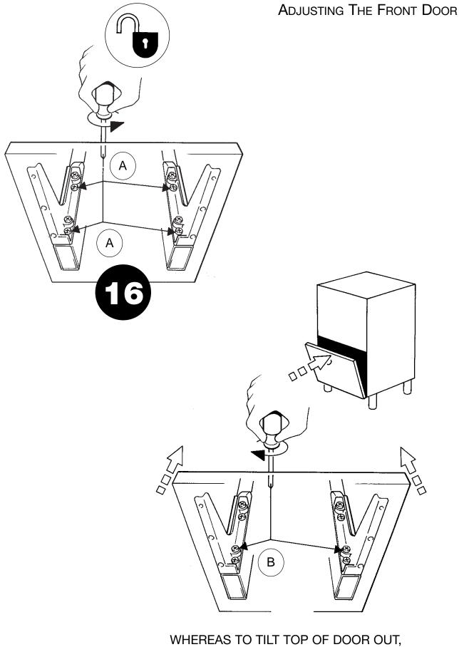
LOOSEN ATTACHMENT SCREWS (A), TIGH-TEN BACK ADJUSTMENT SCREWS (B)
