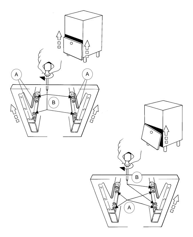
TO RAISE DOOR, LOOSEN ATTACHMENT SCREWS (A) AND TIGHTEN ADJUST-MENT SCREWS (B). TO LEVEL DOOR, RAISE LOW SIDE ONLY UNTIL DOOR IS LEVEL.
