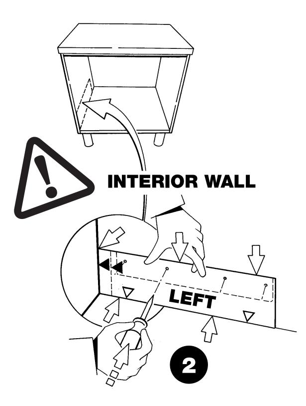
DRILL PILOT HOLES IN EACH SIDE OF CABINET AT LOCATION FOUND BY THE TEMPLATE
