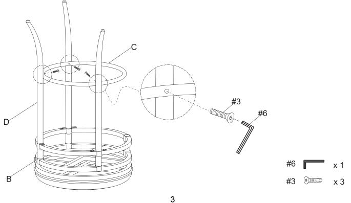
Step 3: Attach remaining leg (part D) to seat (part B) and footrest ring (part C long bolt (part #3), spring washers (part #4), flat washers (part #5) and allen wrench(part #6).
