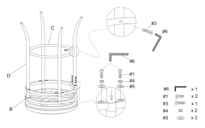
Step 4: Carefully turn the stool over, and attach back (part A) to seat (part B) using short bolts (part #1), medium bolts (part #2), spring washers (part #4), flat washers (part #5) and allen wrench (part #6).
