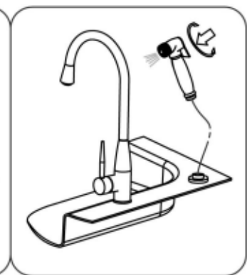
Install 9. Connect and tighten supply hoses to the water supplies. Connect 15 to 9 and the check valve (7). Check for leaks.
