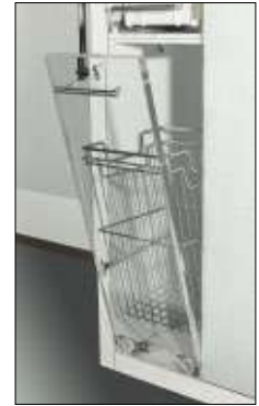
The door is opened by pushing against the door panel. The pressure triggers the release spring in the fitting and the door opens automatically. To close the door, slightly press against the door panel.
