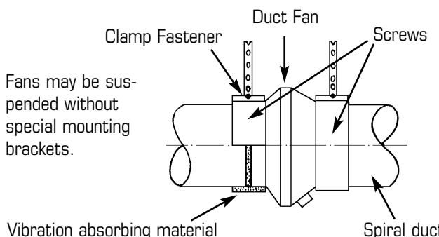
**Mounting Bracket & Screw Locations for FG**
