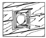
Secure vent cover to wall with 4 SCREWS (included). Caulk around vent cover with a quality caulking compound.
