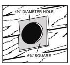
Cut 4½" DIAMETER HOLE all the way through the wall. If wall is not flat: Remove any siding or other outer wall covering from inside 6½" SQUARE - to create a flat surface.
