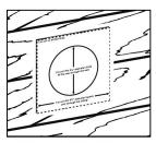
Cut out template below and trace outline on wall. Avoid placement where house wiring or plumbing is located.
