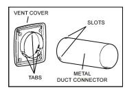
Connect METAL DUCT CONNECTOR together. Snap SLOTS in DUCT into TABS on VENT COVER
