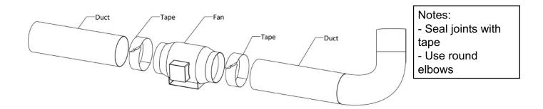
To ensure quiet operation of ENERGY STAR qualified inline and remote fans, each fan shall be installed using sound attenuation techniques appropriate for the installation. For bathroom and general ventilation applications, at least 8 feet of insulated flexible duct shall be installed between the exhaust or supply grille(s) and the fan. For remote ventilation applications, where metal duct is generally required by code, a metal sound attenuator shall be installed between the hood and the fan.
