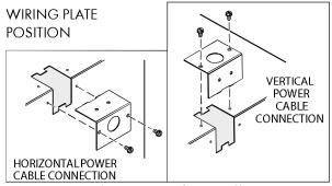
Wiring plate mounts to side or top of housing.
