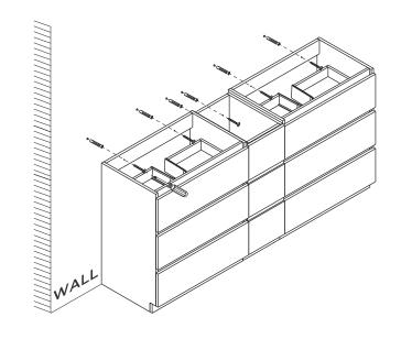
IMPORTANT: Consult an expert for the proper screws/bolts to use when attaching to various constructions, Screws provided do not attach to all wall constrution types. Anchors are not required if brackets are installed in stud.
