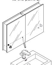
2 Attach bottom bracket (I) to the wall.
