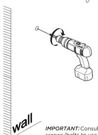
IMPORTANT: Consult an expert for the proper screws/bolts to use when attaching to various constructions, Screws provided do not attach to all wall constrution types. Anchors are not required if brackets are installed in stud.
