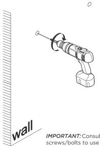
*IMPORTANT:* Consult an expert for the proper screws/bolts to use when attaching to various constructions, Screws provided do not attach to all wall constrution types. Anchors are not required if brackets are installed in stud.
