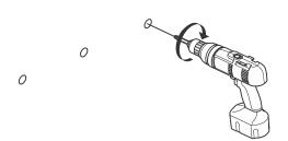
Mark anchor mounting hole locations on wall as shown. Drill holes in the finished wall as required.
