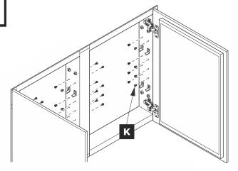
Fill the remaining holes with a plugs (K).
