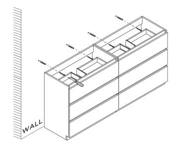
IMPORTANT: Consult an expert for the proper screws/bolts to use when attaching to various constructions, Screws provided do not attach to all wall constrution types. Anchors are not required if brackets are installed in stud.
