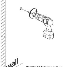
*IMPORTANT:* Consult an expert for the proper screws/bolts to use when attaching to various constructions, Screws provided do not attach to all wall constrution types. Anchors are not required if brackets are installed in stud.
