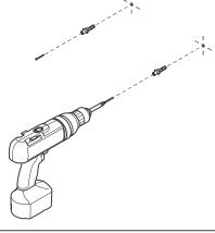
IMPORTANT: Consult an expert for the proper screws/bolts to use when attaching to various constructions, Screws provided do not attach to all wall constrution types. Anchors are not required if brackets are installed in stud.
