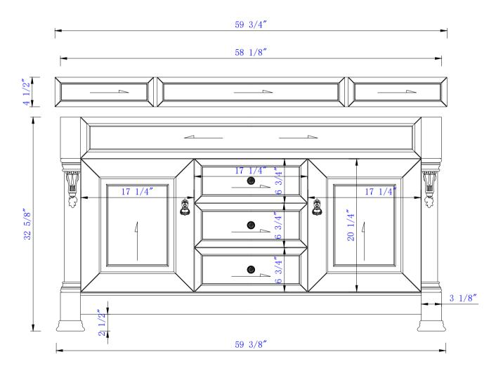
NOTE ONE: Countertops are not shown in these diagrams. (Cabinet Only) NOTE TWO: Wood Backsplash (Shown) is designed for the molding detail to align with sinks in James Martin's Optional Countertops.
