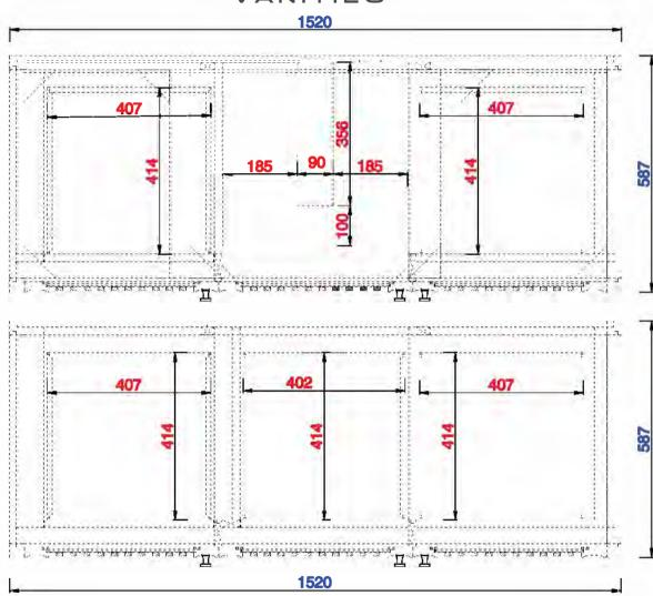
NOTE ONE: Countertops are not shown in these diagrams. (Cabinet Only) NOTE TWO: Internal Shelves (Shown) are designed to align with sinks in la
