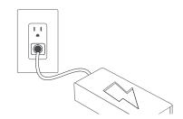
**3.** Plug power supply into switched outlet and turn on Puck Light.
