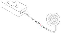
**2.** Insert Male Plug on power supply into Female Plug on Puck Light.
