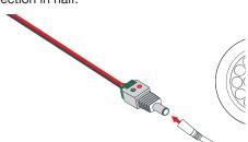
**5.** Insert Male Barrel Connector into Female Plug on puck light.
