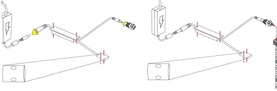
**1.** Insert Male Plug on Power Supply into Female Plug on Door Sensor. Insert Male Plug on Door Sensor into Female Connector on lights.
