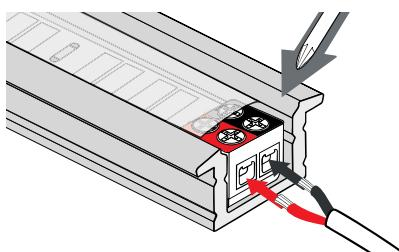
3. Run wires through pre-drilled hole at either end of the groove. Insert stripped wires from power supply or receiver into outer terminals, Red wire to (WW+) side marked in red, Black wire to (CW-) side of tape marked in black; tighten screws.
