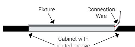
**Wiring for when substrate is thicker than fixture.**
