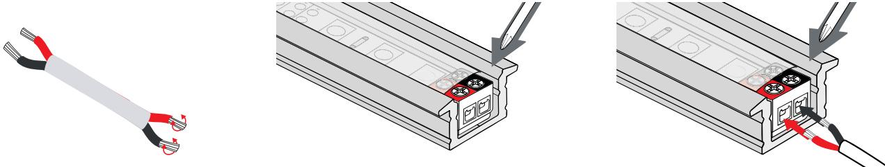
1. Use wire strippers to strip wire 1/4", then twist ends. **NOTE:** wires may be folded over after being twisted, but it is not required.
