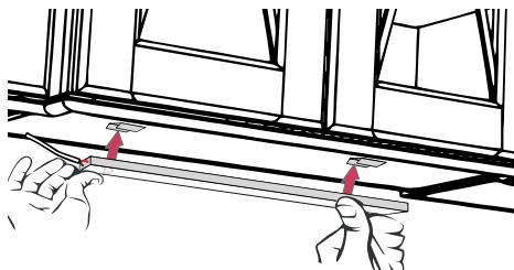
1. Insert fixture up into the groove. Fixture will fit tight. Press along the length of the fixture to ensure fixture is secure in groove.
