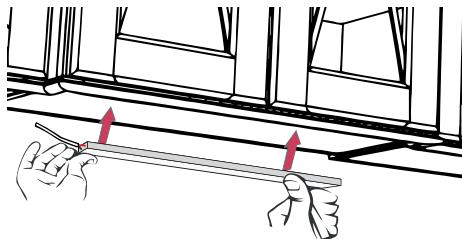
1. Using a 5/8" router bit, hollow out a groove (the length of the fixture) from cabinet or shelf bottom where the fixture will go.
