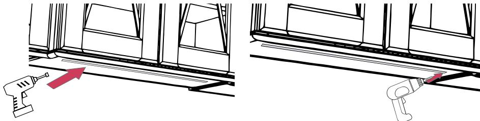
1. Using a 5/8" router bit, hollow out a groove (the length of the fixture) from cabinet or shelf bottom where the fixture will go.
