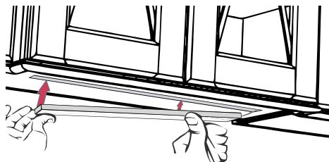
1. Insert fixture up into the groove. Fixture will fit tight. Press along the length of the fixture to ensure fixture is secure in groove.
