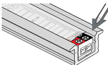
2. Leave frosted lens on the fixture. Use #1 Philips to loosen the 2 outer terminal screws on the 8MM-EZ Connector. **NOTE:** DO NOT loosen the two inner terminal screws.
