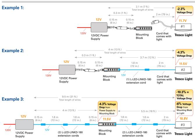
Note: The overall Voltage Drop variance between Light #1 and Light #3 is 8%, which is noticeable
