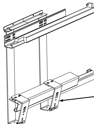
Fold the right side of the slideset up to place inside the cabinet and fold back down to attach to the cabinet floor using the template.
