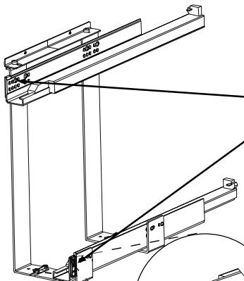
If desired, add spacer using (2) #6 x 5/8" flat head spacer screws to allow the slide to be secured to the face frame for more stability.
