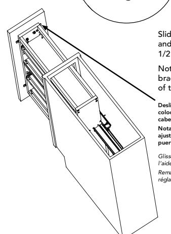
Slide the unit into the cabinet and attach door using (4) #6 x 1/2" flat head screws.
