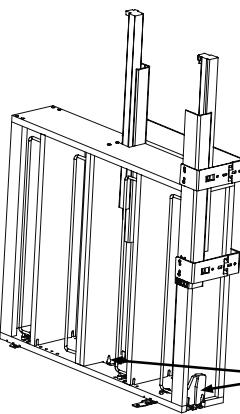
Press orange release levers to disengage slides and pull slides off the unit.
