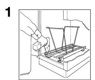
Your RV Series Waste Container has been shipped fully assembled for ease in installation. First remove the container(s) from the wire assembly, place the framework inside your designated space for installation. In the closed position, insert the front 2 screws, making sure the framework is square with the front of the cabinet.
