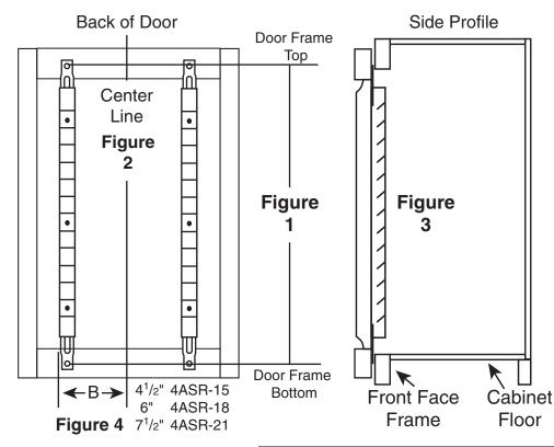
**NEW** mounting brackets adjust up to 5" so they will align in thick portion of door frame. (Standards may have to be cut to fit shorter doors.)
