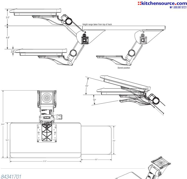
8434D17 Ovation Arm with 6421D Keyboard Tray with Slide-Through Mousing Surface
