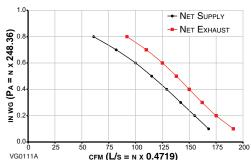
NOTES: Account for an increase in static pressure of approximately 0.2 in. w.g. when installed with the VTY1K1 transition, depending on installation.
