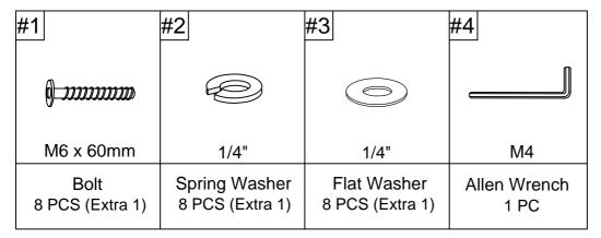
Step 1 . Lay table top (part A) upside down on a soft surface, such as carpet. Attach legs (part B) to table top (part A) using bolts (part #1), spring washers (part #2), flat washers (part #3) and allen wrench (part #4).
