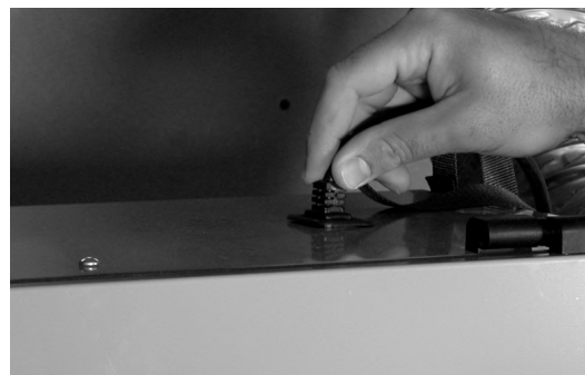
figure 9.1 Insert the power cord on top of the unit. Press firmly to make sure the power cord is secure.
