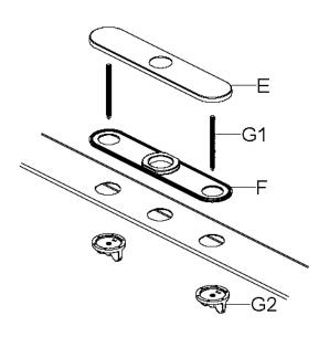
Before installation, remove the flange (D). Screw the bolts (G1) into the escutcheon (E) and ensure that the base plate (F) is pressed onto the escutcheon (E) before the escutcheon (E) is installed over the three holes on the sink. From underneath the sink, hand tighten the mounting nuts (G2). Do not overtighten.
