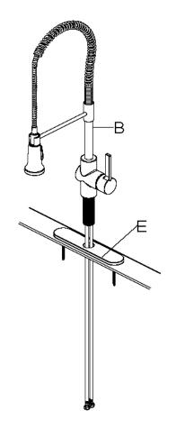
Insert the faucet assembly (B) through the hole in the escutcheon (E).
