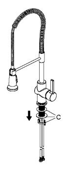
Shut off the water supply. Remove the old faucet. Clean the mounting surface. Remove mounting hardware (C) from faucet body (B).
