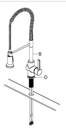
Before installation, ensure that the flange (D) is placed on the bottom of the new faucet assembly (B). Insert the faucet body through the hole in the sink.
