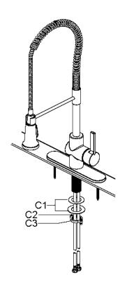
Install the plastic washer and metal washer (C1) onto the threaded mounting shank. Thread the nut (C2) onto the mounting shank. Lock the nut (C2) into position by tightening the screws (C3). Do not overtighten.
