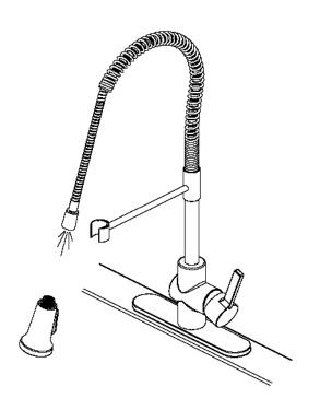
Pull hose assembly out of spout and remove spray head by unscrewing from hose in a counterclockwise direction. Hold the end of the hose down into the sink and turn the faucet on to the warm position. Flush water lines for one minute to flush away any debris. Check for leaks.
