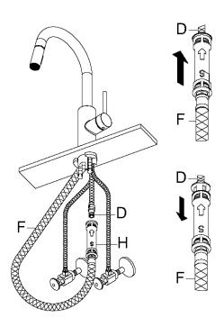
Attach Quick Connect (H) with black end onto spray hose (F) until you hear a click. Attach the other end onto the supply hose (D) until you hear a click.
