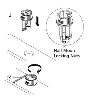
Insert base (J) into sink or countertop with "FR1NT" facing forward. Tighten screws on base (J) with 4mm hex wrench (i2) until base is secure on sink or countertop.
