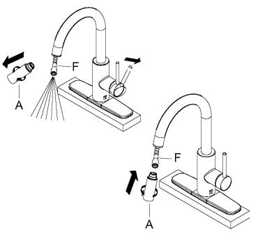
Remove spray head (A). Hold tip of spray hose (F). Turn faucet on for 1 minute to flush any debris. Reconnect spray head (A).
