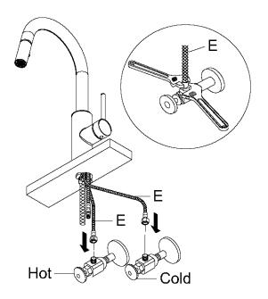
Thread hot & cold waterlines (E) onto angle stops. Tighten with adjustable wrench until snug. Turn on the angle stops and check for leaks.
