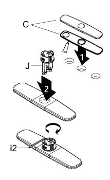
Place a bead of clear silicone sealant (not included) around the edge of the putty plate (C). Secure deck & putty plate (C) on sink or countertop. Insert base (J) into hole of deck & putty plate (C) with "FR↑NT" facing forward. Tighten screws on base (J) with 4mm hex wrench (i2) until base is secure on deck & putty plate (C).
