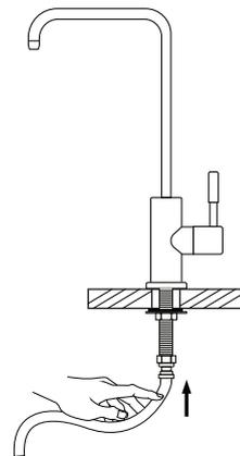
Check for any water leak or kinked hose and correct accordingly.
