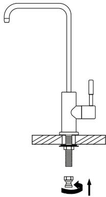
Connect the appropriate connector size. We include a 1/4" and a 3/8" connector. Attached supply hose (not provide with this water tap)
