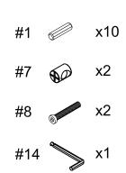
Step 8. Attach front rail (part G) to right partition panel (part F) using large wood dowels (part #1). Attach right panel (part C) to front rail (part G) and bottom panel (part D) using large wood dowels (part #1), barrel nuts (part #7), long bolts (part #8) and allen wrench (part #14).
