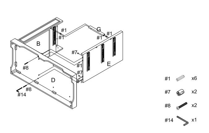
Step 7. Attach front middle rails (part H) to left partition panel (part E) using large wood dowels (part #1). Attach right partition panel (part F) to front middle rails (part H) and bottom panel (part D) using large wood dowels (part #1), barrel nuts (part #7), long bolts (part #8) and allen wrench (part #14).
