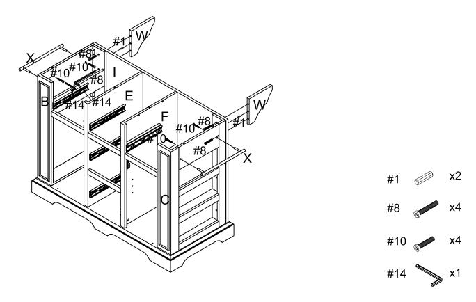
Step 11. Attach top panel (part A) to assembled unit (parts B, C, E, F & I) using large wood dowels (part #1), flat washers (part #12), spring washers (part #11), bolts (part #10) and allen wrench (part #14).
