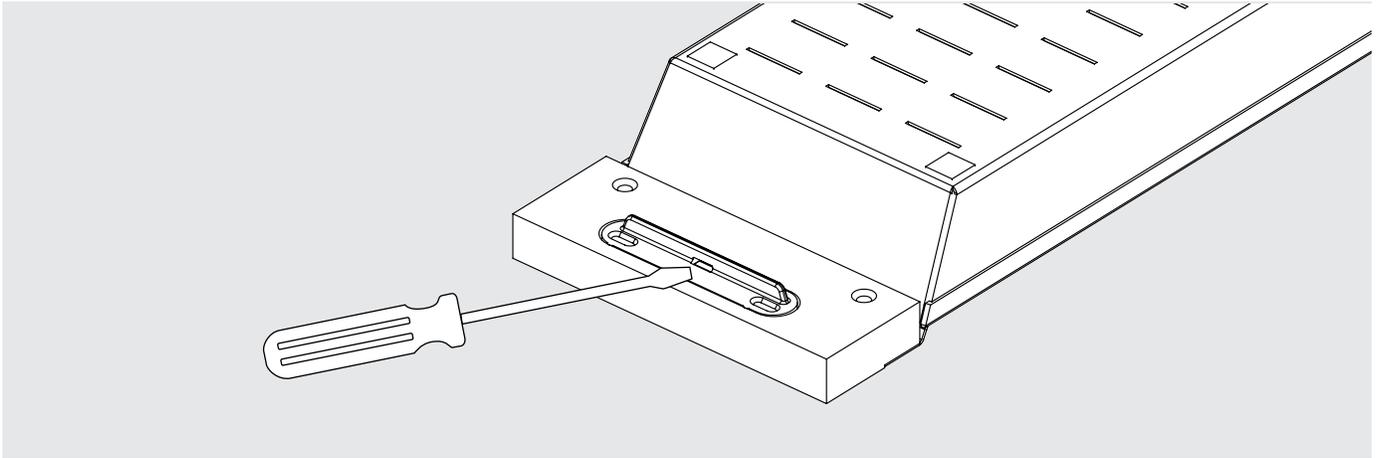
For a flush installation, disassemble only one (1) of the inserts.
