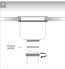
Tighten tail pipe nut to strainer body, ensure the rubber gasket is present.
