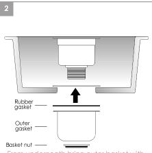
From underneath bring outer basket with rubber gasket under the sink and secure with basket nut.
