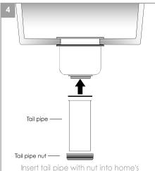
plumbing, then align and secure tail pipe nut to strainer body.
