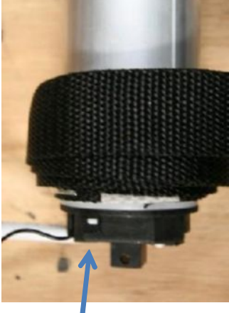
Reset button must use pin, small screw or paperclip to activate. Beeps are very quiet!
