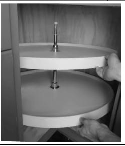
Insert one Shelf Hub through the bottom of a shelf as shown. Place one Shelf Hub Cone on the top of the shelf and fasten using (3) #8 x 1/2" Flat Head Machine Screws provided. NOTE: Make sure the rib inside the Shelf Hub Cone is aligned with the groove in the hub (see picture). Repeat with second shelf.
