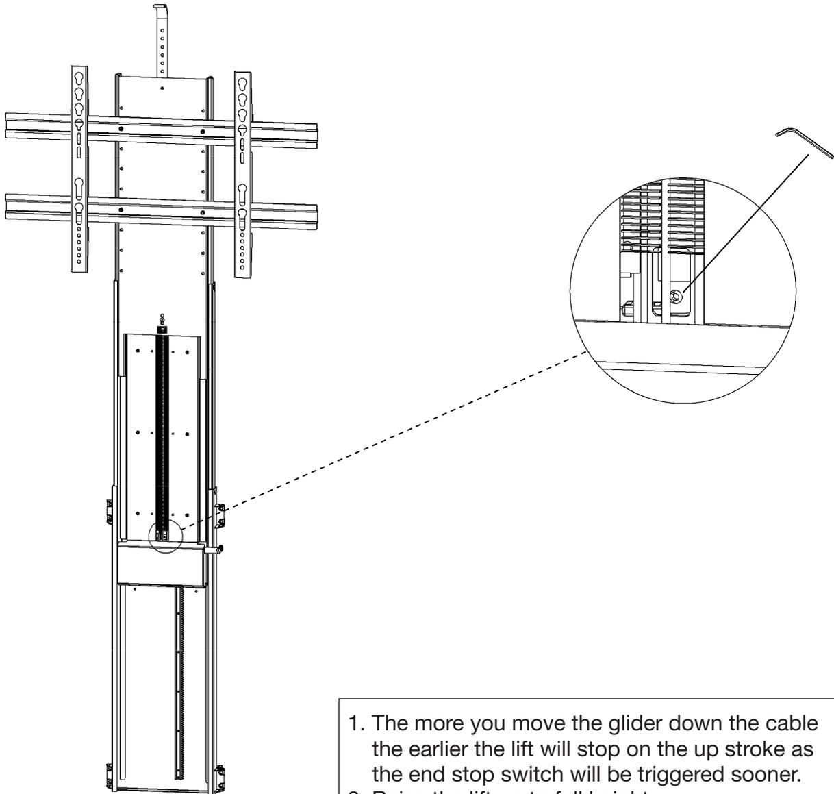
1. The more you move the glider down the cable the earlier the lift will stop on the up stroke as the end stop switch will be triggered sooner.
