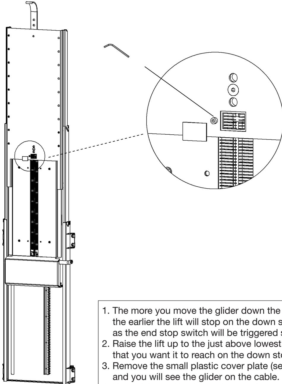
1. The more you move the glider down the cable the earlier the lift will stop on the down stroke as the end stop switch will be triggered sooner.
