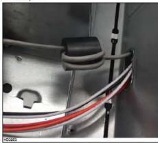
Open the provided connection box. Using long nose pliers, break away 2 cable entry notches on the lid (one per side).
