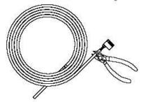
• Run one end of the ADA cable through the range hood wire clamp, along with the power cable, giving enough lenght to make the connection inside the box. Tighten the wire clamp, then strip the end of the 3 wires from provided ADA cable.
