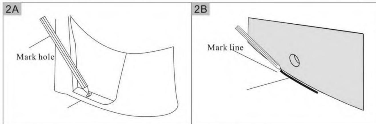
2. Put the water closet onto the installing position. Make sure the + centre lines of floor and water closet are aligned. Then mark the installing holes with pencil.
