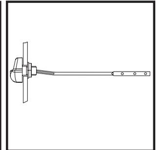
Enter the nut on the handle and tighten.
