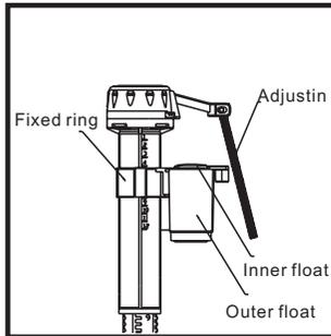
Pull the adjusting rod, and raise or lower the fixed ring to the desired water level.
