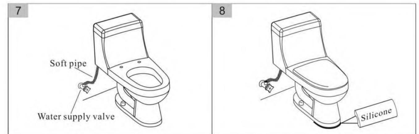
7. Install the water supply valve, then connect the filter and water supply soft pipe of cistern. Check the connection carefully to make sure there is no leakage.
