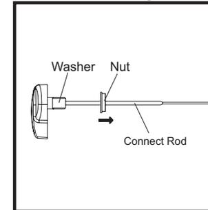
Loose the nut clockwise take away the nut and the washer from the rod.
