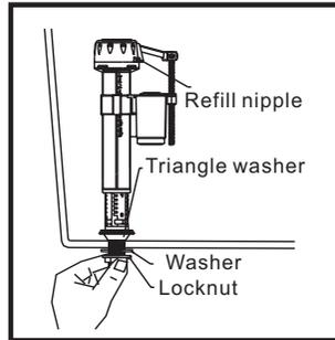
Unscrew the locknut and washer. Position the fill valve into the tank, then screw the washer and locknut.
