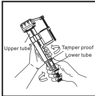
Take off the tamper proof, and adjust the height by screwing the upper and lower tube. Then fix the tamper proof.
