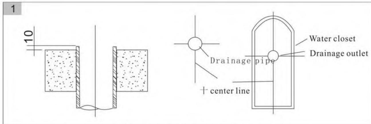
1. Mark the + centre line according to the drainage outlet on the floor and the one of the water closet.
