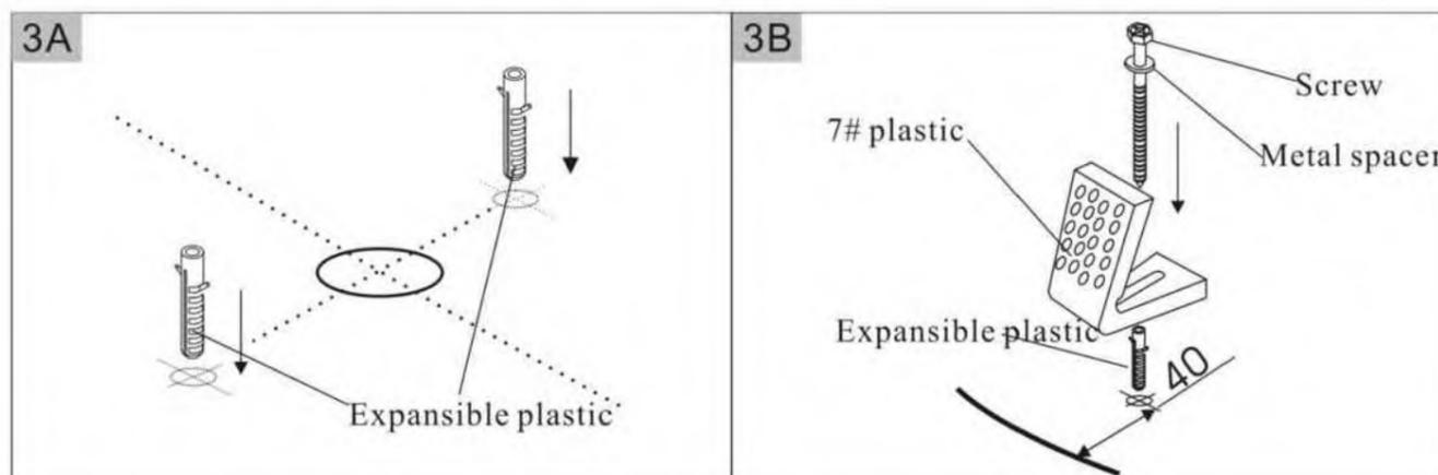
3. Remove the product and drill holes according to the marks. Then insert the plastics.
