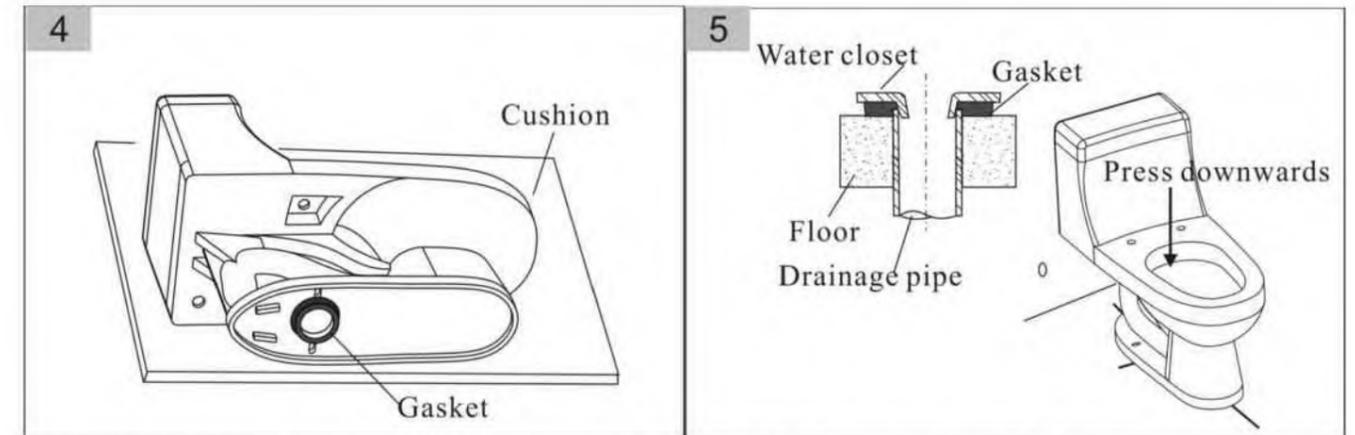
4. Put the product onto the cushion flatly, then cover the gasket onto the drainage outlet tightly.
