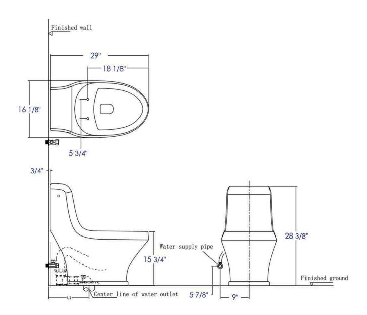
Note: All product dimensions are approximate and should be verified on site prior to installation.
