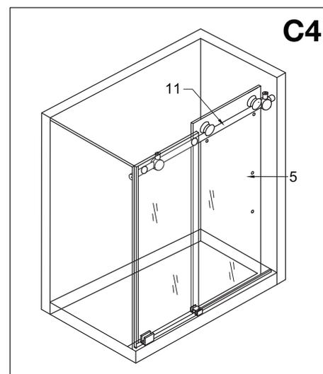
5. Verify that the bottom of the door rests in the back notch of the bottom door guide (#8). /
