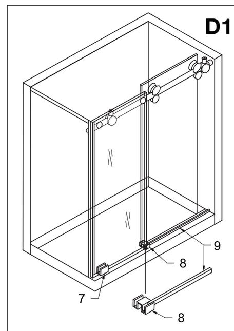
9. Remove the threshold. Apply silicone to the underside of the threshold. Place the threshold back onto its shower base around the inside and outside of the shower base. Remove any excess silicone from the threshold. /
