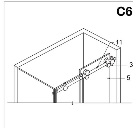
7. Adjust the stoppers' (#10) position on the structural rail and tighten the hex screws. Position the stoppers in a spot on the structural rail that will avoid the handle from hitting the glass when the door is in an open position. /
