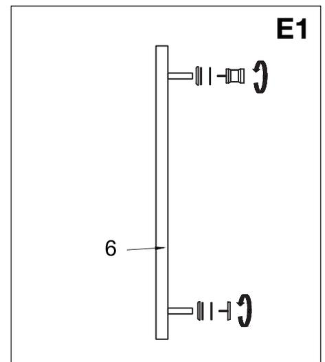
2. Place the handle to the position on the door. Place plastic washers (supplied) on each side of the door. /
